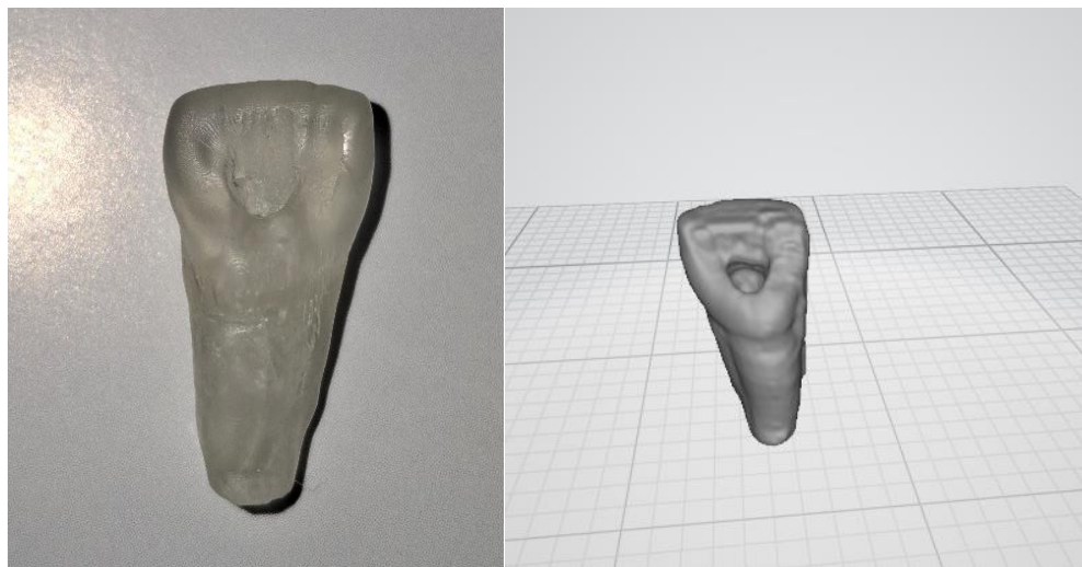
Figure 2. STL output of the tooth model (right) along with the resin-printed tooth model (left)
